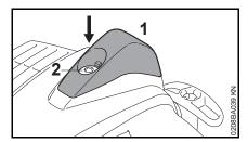
• Fit the cap (1), insert the screw (2) and tighten it down firmly.
