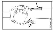
Depress throttle trigger lockout and pull the throttle trigger – the choke knob moves to the Run I position.
