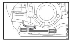
Check the pickup bodies in the fuel tank annually and have them replaced when necessary
